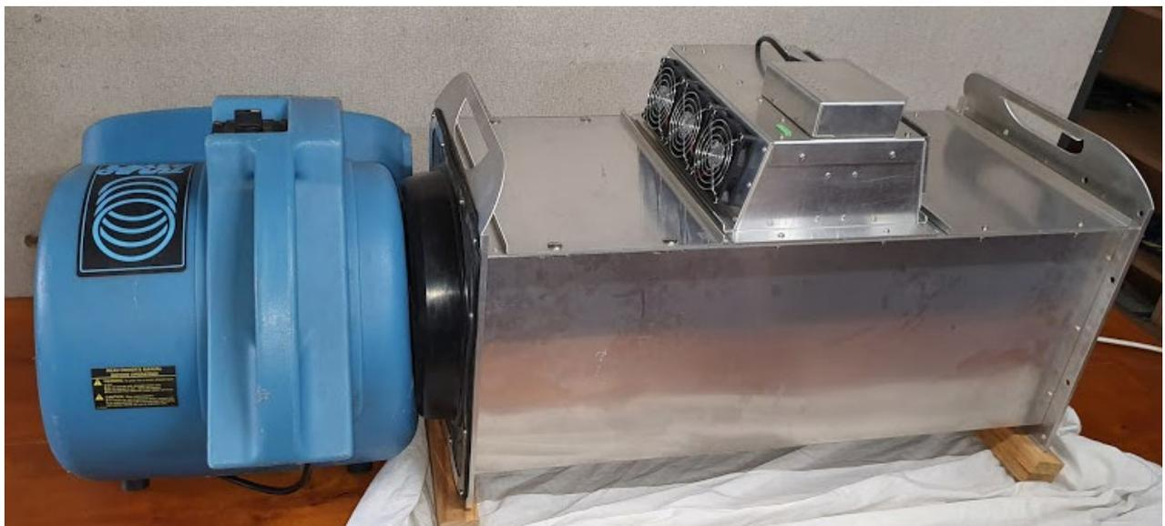
5 Optic unit with blower/air mover that will provide a directed stream over the area to be treated.
